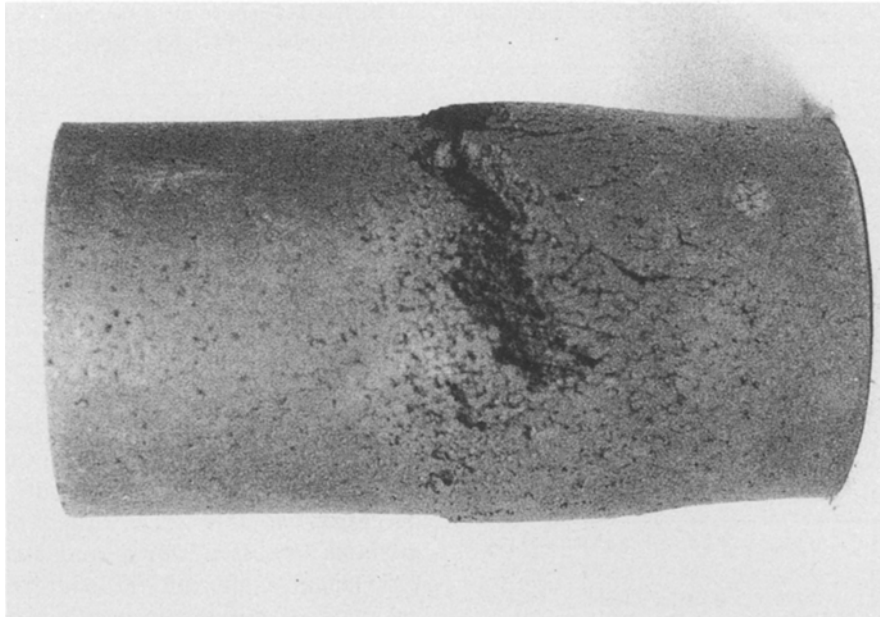
Figure 8 Cylindrical specimen showing microcracks and mode of failure.
